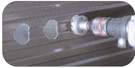
PERFORMANCE COMPARISON NEW CT5 to PREVIOUS CT5 (2") Material: SUS304 Stainless Steel Material thickness: 1/8" - Speed: 800 rpm
