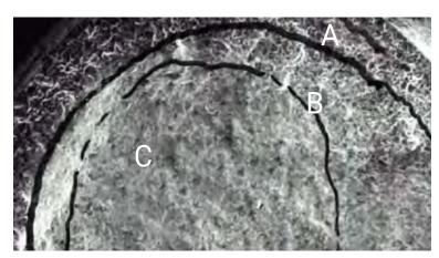
In case hardened fasteners, only the brittle outer layer is vulnerable to HASCC. However, a weakening outer layer placed the entire load onto the core of the fastener, a significantly smaller diameter of steel than the original design. The design load can overwhelm this reduced fastener diameter, leading to failure.
