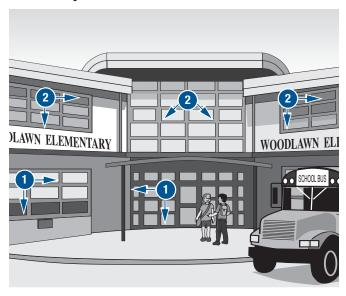
1 FOR DOOR AND WINDOW PERIMETERS UP TO 10 FEET ABOVE GRADE - Pecora Dynaflex. 2 FOR DOOR AND WINDOW PERIMETERS OVER 10 FEET ABOVE GRADE - Pecora Dynafrol II.
