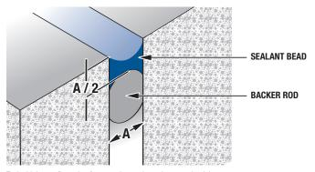
Typical joint configuration for a moving or dynamic expansion joint
