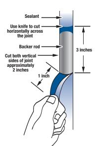
All surfaces must be clean. sound and free of surface water. Remove laitance, curing coatings, compounds. grease, rust, waxes, and other bonding inhibiting substances. Application over paints or coatings is not recommended unless the paint or coating can relied upon to impart adhesive properties equal to the sealant/virgin concrete bond and maintain the security properties needed.
