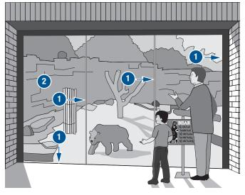
1 GLAZING JOINTS - Pecora Dynaflex or Pecora Dynaflex SC. 2 NON-MOVING FEATURES - Dynapoxy EP-1200.
