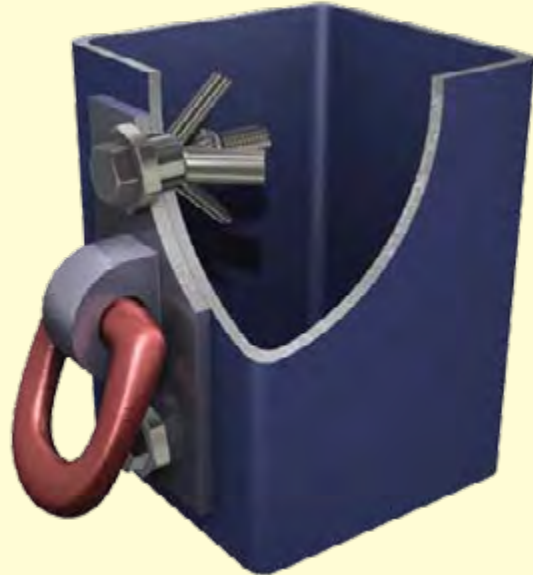
Rigging point to outside of hollow section
