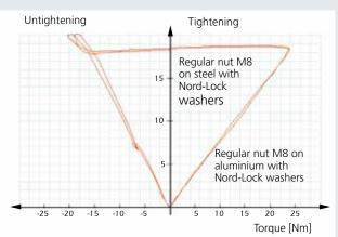
When using Nord-Lock washers, sliding always occurs between the upper washer and the bolt head / nut. At a given torque, the preload will be the same, regardless of the contact material.
