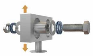
Fig 2: Drawing of the test rig. The assembled parts are vibrated vertically and the joints are subjected to two impacts per cycle. The impacts are parallel to the bolt. The arrow displays the direction of vibration during the test. After testing, the fasteners are inspected for rotation.
