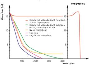
Fig 1: The Junker test shows that Nord-Lock washers safely secured the bolted connection; only a limited amount of tension is initially lost due to normal settlements. The wedge-locking function is verified through the clear increase in tension during untightening. All other bolt locking methods in the test failed to prevent loosening of the joint.
