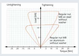
When no washer is used under the fastener, the friction depends on the contact surface. At a given torque, the obtained preload will vary depending on the contact material.
